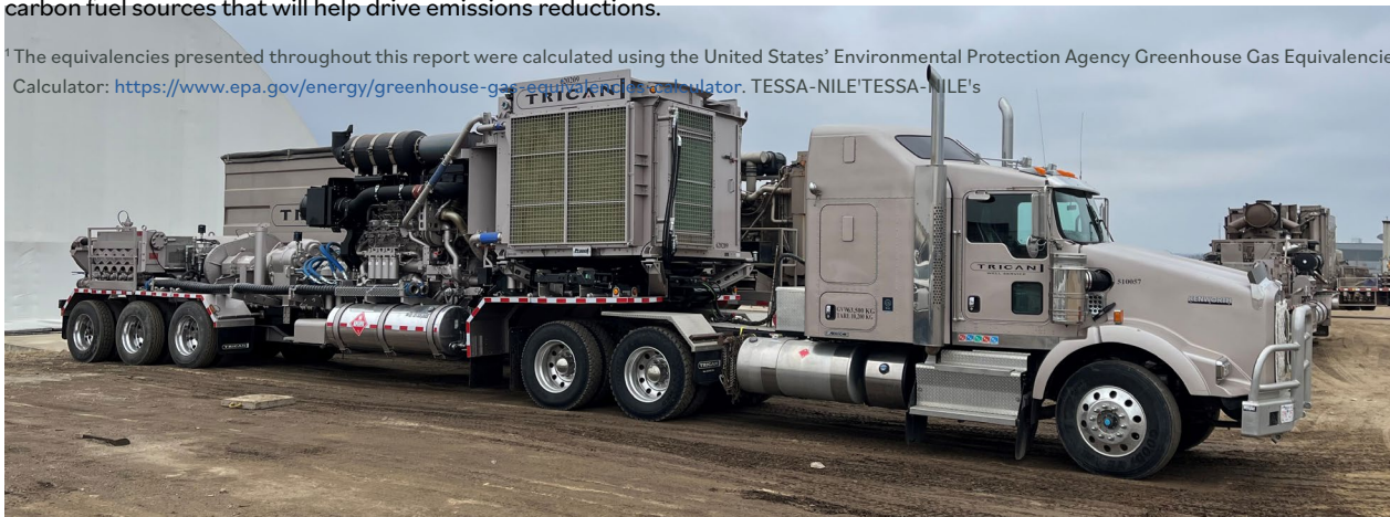
Photo: TESSA-NILE Tier 4 DGB Hydraulic Fracturing Engine
