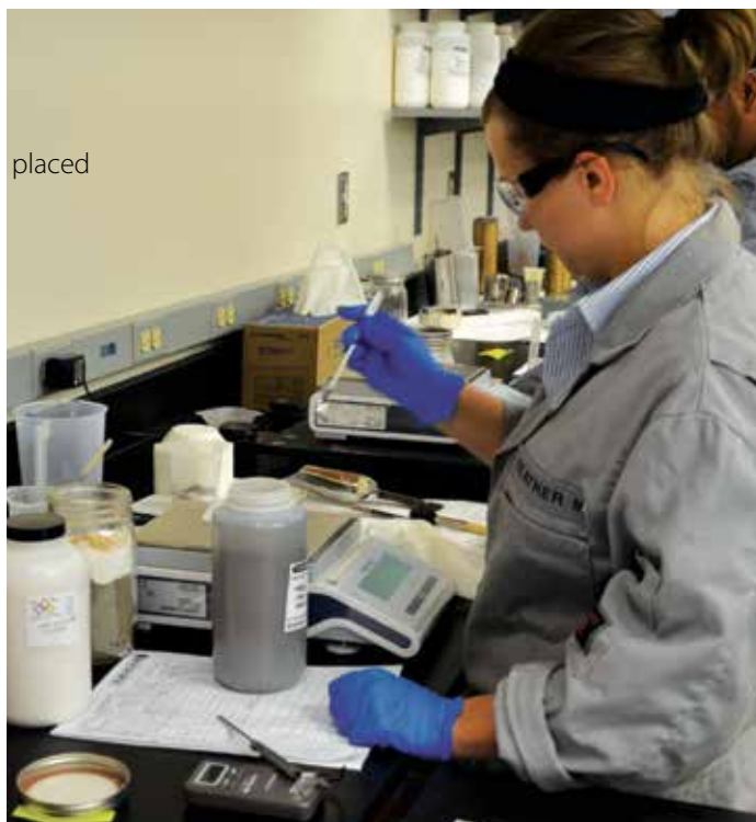
Preparing a cement blend for testing.
